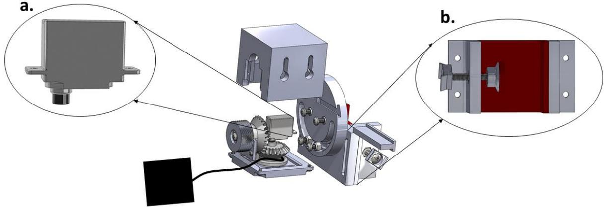
**Figure 1.** 3D solid model view (exploded) of the skin stretch device. a) Nano servo motor fixed to a bevel gear and a disc used to pull on a thread attached to elastic sports tape. b) 3D printed clamp used to affix the skin stretch device to a chair.
