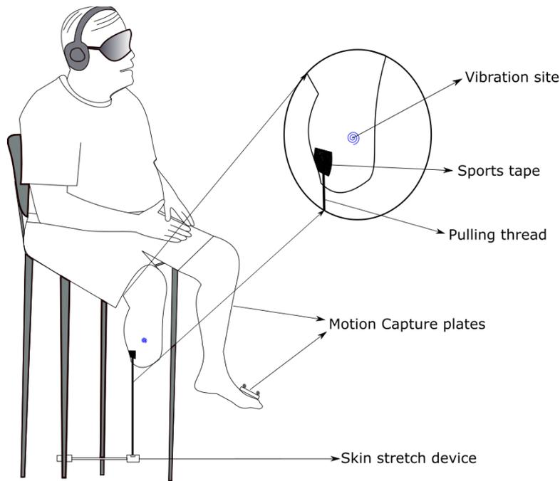
**Figure 2.** Experimental setup. Participant sitting comfortably on a high chair during a vibration and skin stretch trial.
